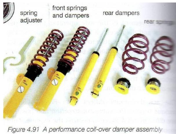
Figure 4.91 A performance coil-over damper assembly
