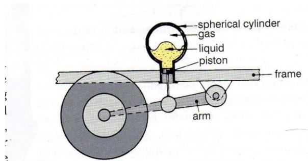
Figure 4.80 A hydro-pneumatic suspension system
