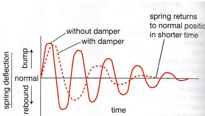
Figure 4.87 Spring oscillation curves
